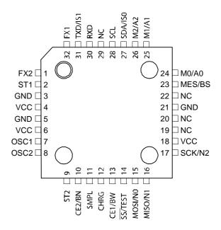
NOTE: Bottom Pad for MLF Package Should be Soldered to Ground.
