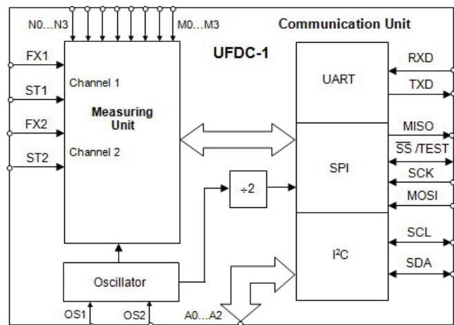
The UFDC-1 can be easily included into digital environment, controlled by an external microcontroller (slave mode) or work independently as a separate measuring unit without an external control (master mode). The function selection can be configured in both software and hardware.
